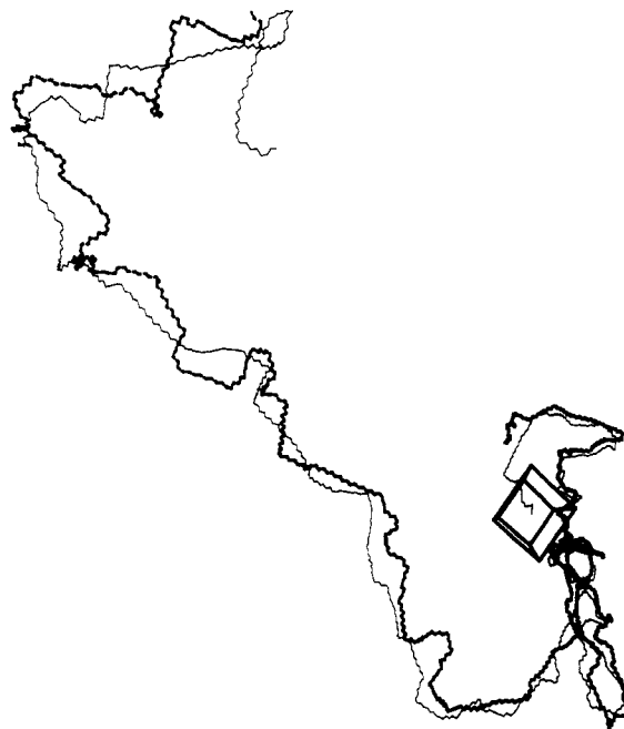
Figure 2. Comparison of the chain structure for one sample before (thin line) and after (thick line) heat treatment. Only the coordinates of the continuous primary chain have been shown in both cases. The periodic MD cell which is filled by images of the primary chain is also shown.
